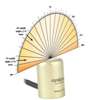
Directional, or cosine, response is defined as the measurement error at a specific angle of radiation incidence. Error for Apogee SQ series quantum sensors is approximately  $\pm 2$  % and  $\pm 5$  % at solar zenith angles of 45° and 75°, respectively.
