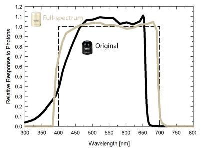
Mean spectral response measurements of six replicate Apogee SQ-100 (original) and SQ-500 (full-spectrum) series quantum sensor. Spectral response measurements were made at 10 nm increments across a wavelength range of 300 to 800 nm in a monochromator with an attached electric light source. Measured spectral data from each quantum sensor were normalized by the measured spectral response of the monochromator/electric light combination, which was measured with a spectroradiometer.
