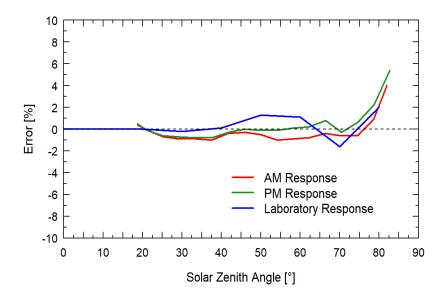
Mean cosine response of seven apogee SQ-500 quantum sensors. Cosine response measurements were made on the rooftop of the Apogee building in Logan, UT. Cosine response was calculated as the relative difference of SQ-500 quantum sensors from the mean of replicate reference quantum sensors (LI-COR models LI-190 and LI-190R, Kipp & Zonen model PQS 1).
